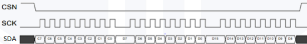
Figure 8.4.3 wire SPI write operation
