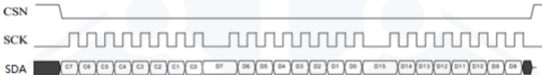
Figure 8.3.3 wire SPI read operation
